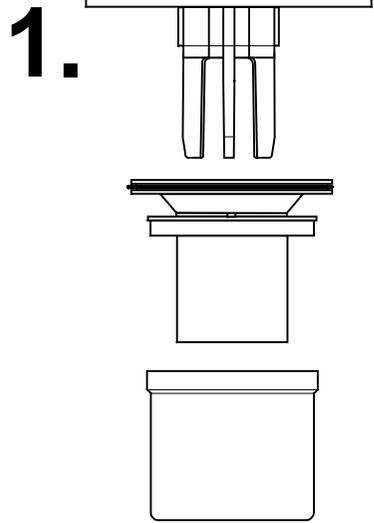
The Trap provides a flow rate of 34 litres per minute when tested in accordance with EN274-2:2002. The flow rate can be seriously impaired if an adequate fall is not maintained throughout the length of the waste pipe.
