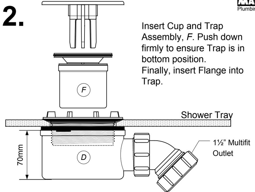
Insert Cup and Trap Assembly, F. Push down firmly to ensure Trap is in bottom position. Finally, insert Flange into Trap.
