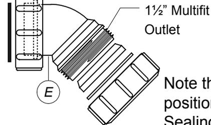
Note the order and position of the Sealing Washers. Failure to do so can result in water leakage.
